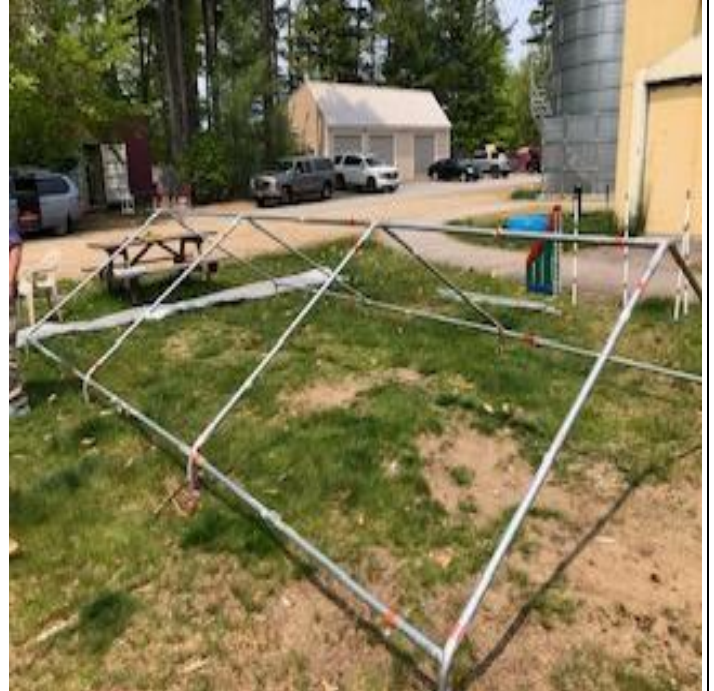
Two-section roof assembles the same, just one less roof section in the frame.
